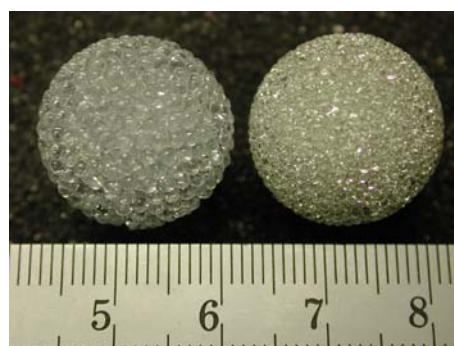
Fig. 8 Porous glass spheres made with 1.5 and 0.8–1.2 mm of beads
